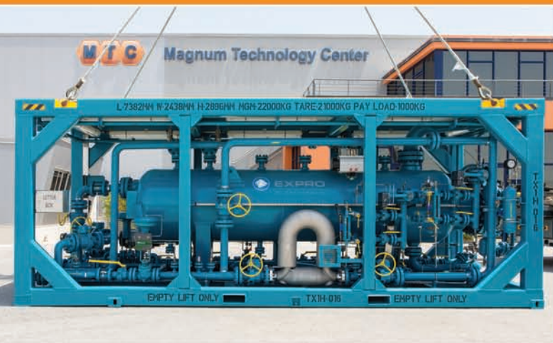
1440 Psi NORSOK Separator in offshore DNV frame
