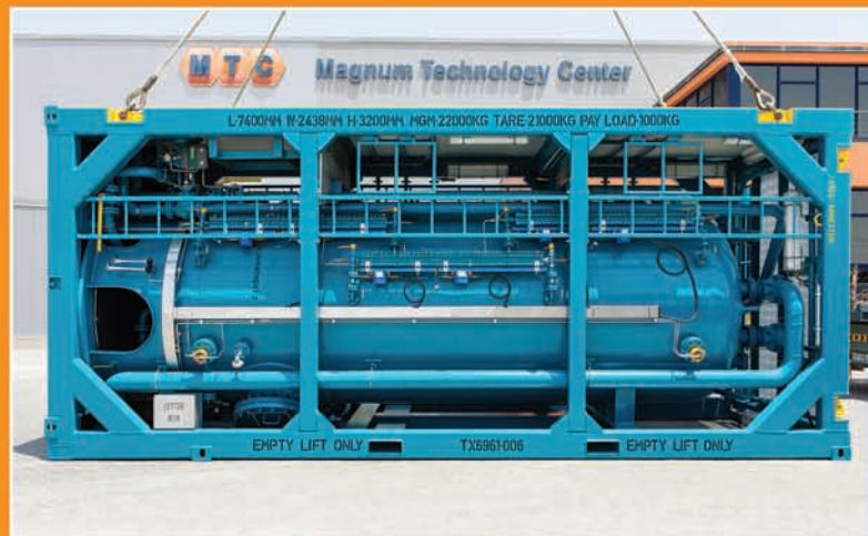
250 Psi 100 Bbl NORSOK Surge tank in offshore DNV frame
